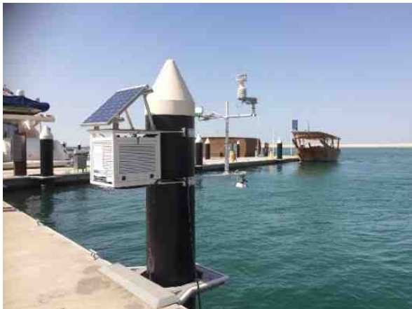
TideStation with VRS-20, Pressure and METPak with Solar Charging
