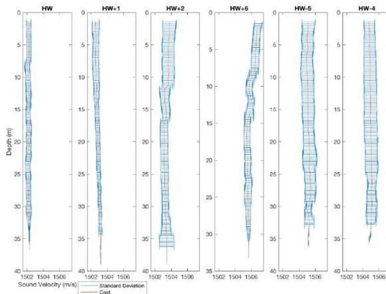
Figure 8: Block variance (deepest cast compared to all other profiles within block)
