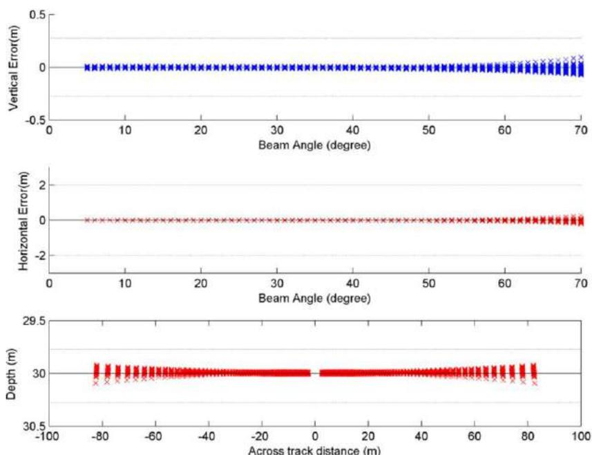
Figure 9: Ray tracing errors for HW (dashed lines represent IHO special order limits)
