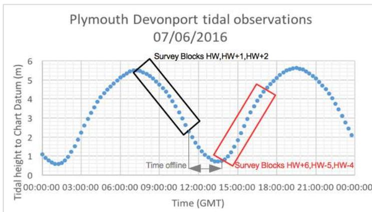
Figure 5: Data acquisition periods showing survey blocks completed through the tidal cycle
