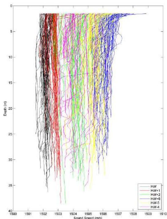
Figure 7: All the sound speed profiles, colour coded by survey block
