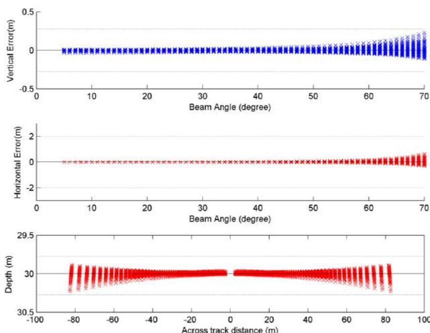
Figure 10: Ray tracing errors for HW+6 (dashed lines represent IHO special order limits)
