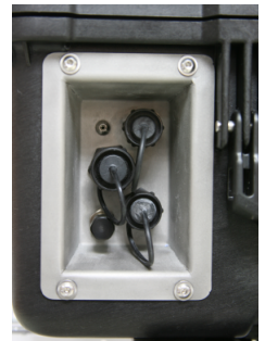
TideStation Portable - recessed connector bay
