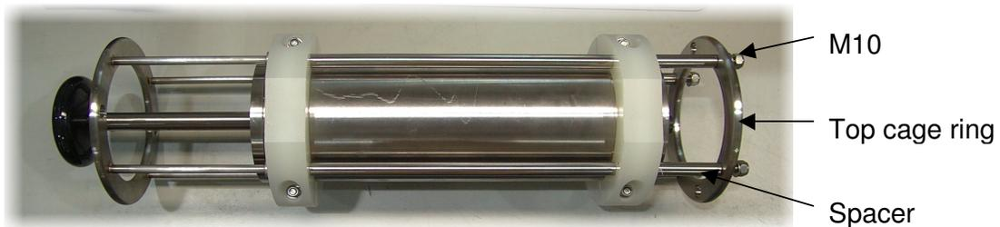
2. Lift the instrument out of the cage, complete with the polypropylene mounting brackets. Take care to catch the central spacer tubes as you lift.
