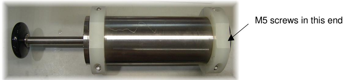
4. Without twisting or putting undue stress on the Subconn connector slide the bulkhead and attached battery pack out of the main housing. A slot between the tube and the bulkhead allows levering with a screwdriver if necessary. Take care not to scratch the bore of the tube.
