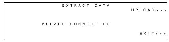
Connect the unit to a PC via the data interface lead supplied. Run a terminal emulation program on the PC, ensuring that communications are correctly set to 4800 baud, 8 data bits, 1 stop bit, no parity bits, flow control NONE. If the data is to be saved on the PC, make sure that the data is directed to a file name. It is uploaded as a text file, with "Tab" delimiters, so it can be read into a word processor or spreadsheet application.
