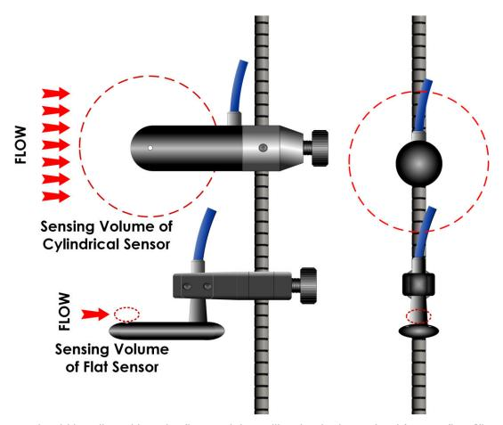
The sensor should be aligned into the flow and the calibration is determined for +ve flow [flow on to the sensor at the electrode end] with the sensor upstream of the wading rod.
