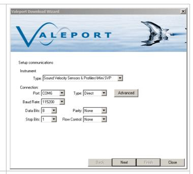
Ensure the instrument is switched on and connected. Extend the interrupt timeout if the unit is operating in burst mode (or cycle the power to the instrument)
