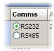
This is because Valeport uses a half-duplex RS485 method, where the same wire pair is used to both transmit and receive data. For this reason, both the instrument and the PC must allow a short delay between transmitting and receiving data; such a delay is not necessary for normal RS232 communications.
