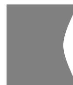
These rings should be fitted into the o-ring groove on the “dry”, or low pressure side of the o-ring, with the concave surface adjacent to the o-ring itself:
