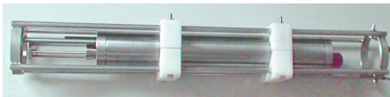
Slide the instrument out of the cage, in either direction.
