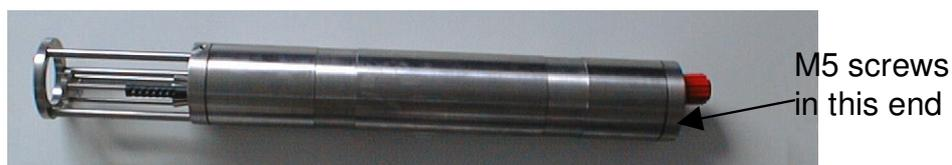
2. Remove the 3 M5 x 20 socket cap screws in the connector bulkhead, using the Allen key provided. Note that these screws are titanium, and should be replaced with titanium screws if lost. Other materials may suffer galvanic corrosion and may be destroyed.
