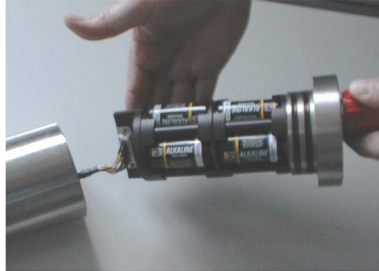
4. A lead connects the battery pack to the electronics inside the tube. This may be disconnected at the battery pack if required, for ease.
