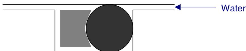
It is particularly important to note that in order to fit these rings, they must be stretched slightly to pass over the instrument body. This stretch does not immediately recover, with the result that the AE ring may not sit snugly in the groove at first. Fitting the tube to the instrument at this point may result in the AE ring riding out of the groove, and preventing a proper seal. The instrument may then leak.
