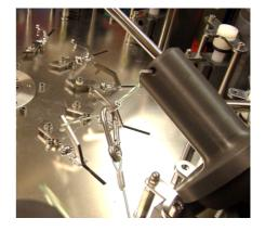
Finally, to prepare the bottle for deployment, ensure that the tap on the side of the bottle is pulled out as far as the stop will allow, and that the release screw on the top of the bottle is tightly secured.
