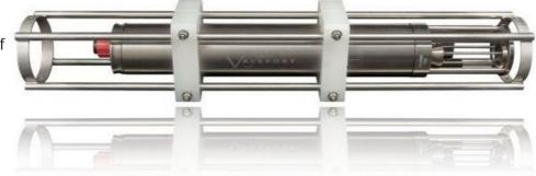
2. Slide the instrument out of the cage, in either direction.
