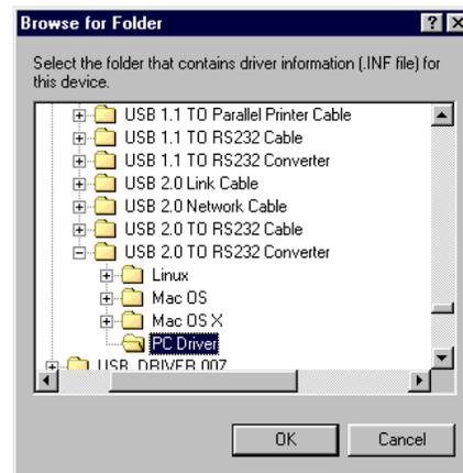
Locate the folder that contains the driver and click OK. Note that the driver may be supplied on a separate disk to the main WaveLog Express program, but nevertheless will be under the USB 2.0 to RS232 Converter \ PC Driver directory as indicated above.
