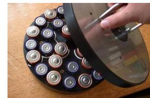
5. Note that the lower half of the carousel is marked with white lines. These indicate the boundaries of each of the 4 banks of 8 cells. Since these banks of cells are all connected in parallel, it is possible to fill 1, 2, 3 or all 4 banks – obviously a partially filled carousel will offer decreased operational time, but may be financially beneficial for short term deployments. Insert the cells into the required holes, taking care to observe the correct polarity.
