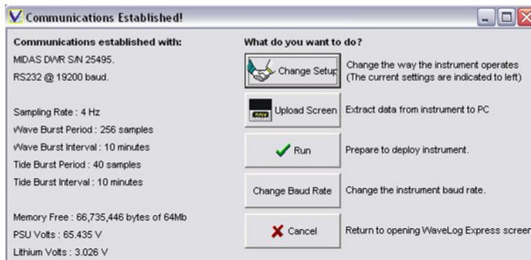
Once communications are successfully established you will see the following screen. This allows you to change setup, upload data, run the instrument or change the baud rate.
