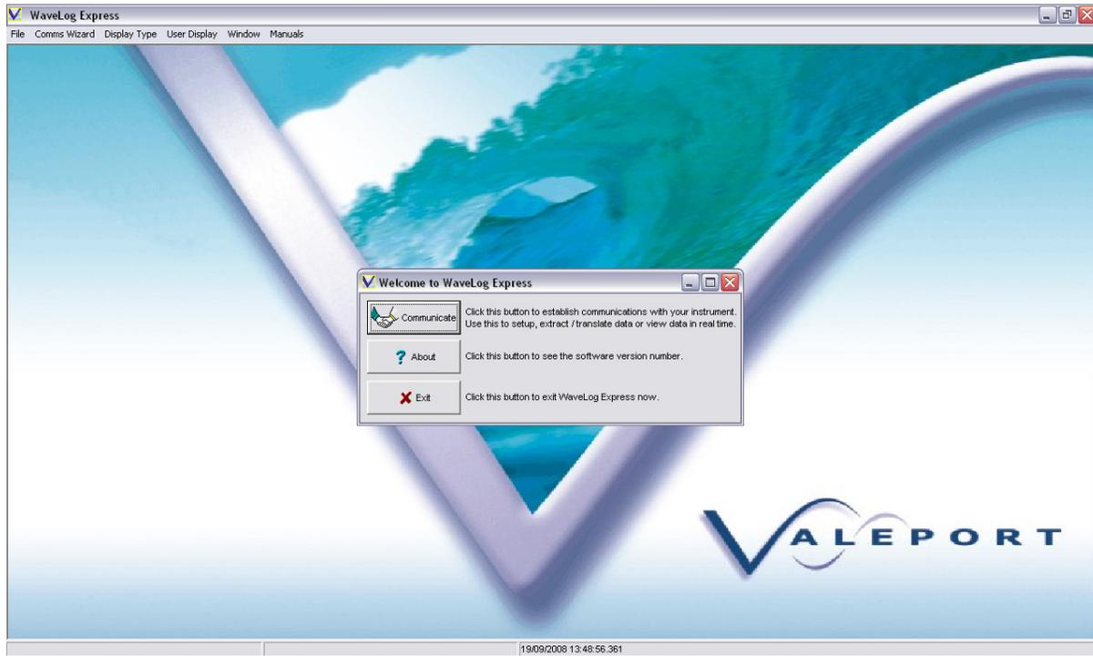
This page is the main operating environment for the WaveLog Express software – all command and data display windows are opened within this area, as described in subsequent sections. Key features are the menu bar at the top, and the status bar at the bottom. There are three sections to the status bar:
