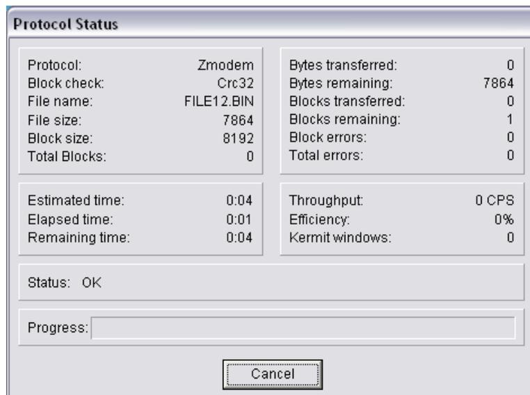
Data will be automatically uploaded into a subdirectory of the WaveLog Express directory, labelled according to the serial number of the instrument and the date of upload (Please see Section 5.6). This subdirectory will be created if necessary. The following screen will be shown:
