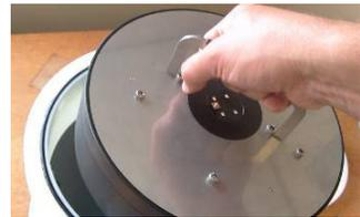
4. To open the battery carousel, remove the five M5 screws as indicated. The carousel will then separate into upper and lower halves, exposing the batteries themselves.
