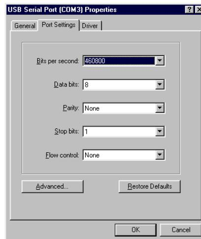
Ensure that the settings are as shown above; this will optimise the port for use with the Wave Recorder. Finally click the Advanced button.
