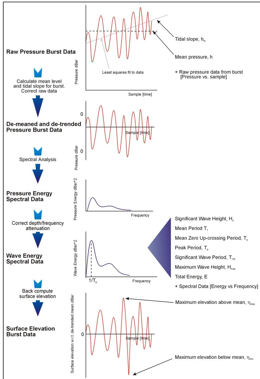
Level and height units are all logged and calculated in pressure dBar, which may be converted to depth using the following relationships:
