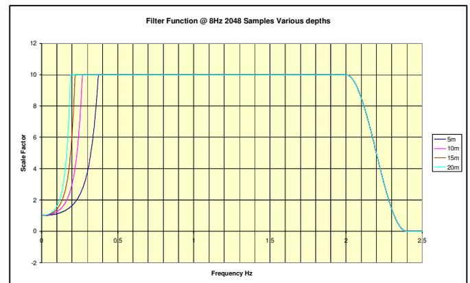
Below is a plot showing the wave frequency at which the scale factor is capped (i.e. reaches a value of 10), at different deployment depths.
