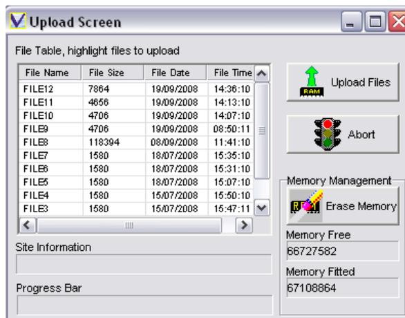
**File Name** This is automatically generated by the instrument, in the form FILE#, where # is the next number in sequence. There is no limit to the maximum number of files that can be stored, apart from the physical capacity of the memory.
