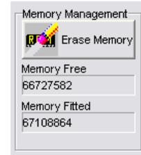
Take care when erasing memory. Although the user is asked twice for confirmation, they should ensure that all required data has been uploaded prior to erasing the memory.
