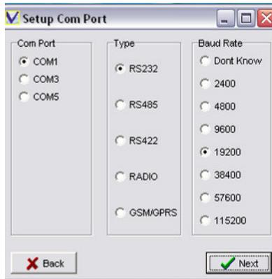
Begin by selecting the correct comm port, communication type and required baud rate.
