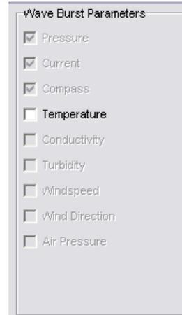
In this example, the device (a MIDAS DWR) is only fitted with the standard temperature sensor in addition to the pressure, current and compass sensors, so only that sensor is shown as available.
