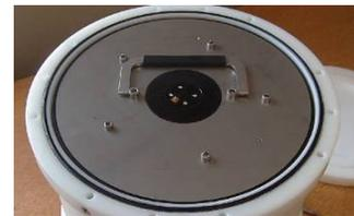
3. To remove the battery carousel, simply lift the stainless steel handle to a vertical position, and pull; the carousel will lift out of the instrument. If a spare preloaded carousel is available, please proceed to step 7.
