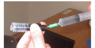
Note that this procedure should be carried out as close as possible to the actual deployment time. Once submerged, the water pressure will prevent the oil from leaking out of the silt trap assembly. Whilst it is held in place by capillary action, the oil is more likely to leak out of the silt trap if the instrument is in the air.
