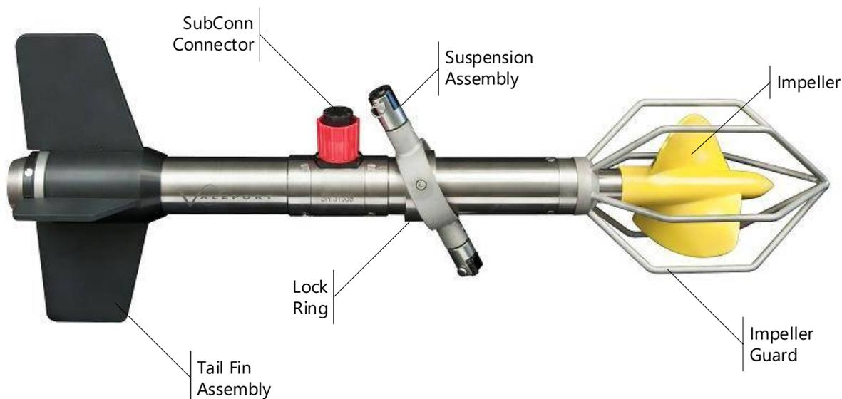
The instrument is provided with a suspension assembly for users to attach to a suspension or mooring line. If the Valeport polyurethane covered multi-core cable is being used, then this has a maximum working load of 100kgf, and if a sinker weight is being used, it is important that this load is not exceeded.
