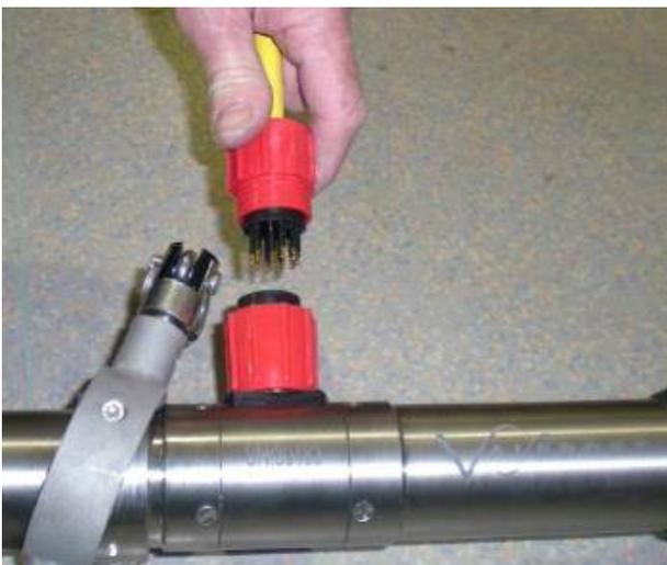
When deploying the unit in self-recording mode, the SubConn switch cap will need to be attached in place of the communication cable
