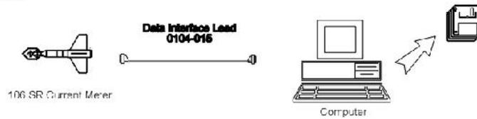
Figure 2: Model 106 Sensor Layout
