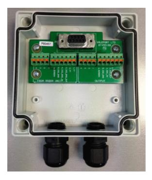
The bare cable from the VRS-20 should be passed through the cable gland and terminated in the push fit connectors with reference to the wiring schedule.
