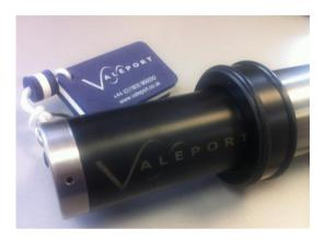
The Bluetooth miniLogger is rated to 2000m and is secured using the same lock ring as used by the standard logger pack.
