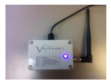
The receiver will install as a USB serial port adaptor and should install automatically on most windows PC's. If the receiver will not automatically install, drivers can be downloaded from:
