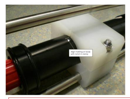
If the instrument is removed from the deployment cage for any reason, it should be reinstalled securely, taking note of the alignment markings on the housing (see photo) and polypropylene clamp
