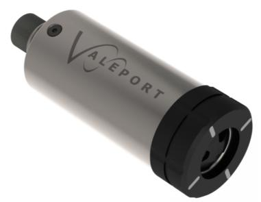
The pressure sensor fitted to the ultraP is a temperature compensated piezo-resistive sensor, which delivers the performance previously only available from a resonant quartz sensor at a more cost-effective price.
