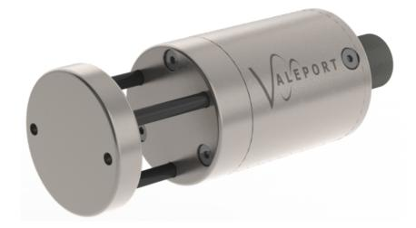
Each sound velocity measurement is made using a single pulse of sound travelling over a known distance, so is independent of the inherent calculation errors present in all CTDs. Valeport's unique digital signal processing technique virtually eliminates signal noise errors, and gives almost instantaneous response available; the digital measurement is also entirely linear, giving predictable performance under all conditions.
