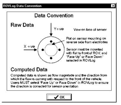
This shows that looking at the face of the sensor, with the instrument mounted face up, +ve Y flow is into the vehicle, and +ve X flow is from left to right.
