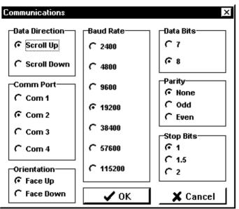
The Model 803 default output format is 19200 baud, 8 data bits, 1 stop bit, no parity bits. The user should check that the format has not been changed, and select the correct comm port and whether they wish to see data scrolled up or down. Finally, it is vital to set the orientation of the sensor correctly (Face Up or Face Down). Setting this wrongly will result in incorrect bearing data. When all settings are correct, press OK.
