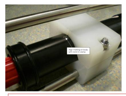
If the instrument is removed from the deployment cage for any reason, it should be reinstalled securely, taking note of the alignment markings on the housing (see photo) and polypropylene clamp
