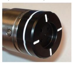
The pressure tare should be taken with the sensor in the same orientation as it will be deployed (horizontal, pointing up or pointing down) to negate any effects of the weight of the sensing element itself. Whilst this effect is small, it is an unnecessary contribution to the error budget.
