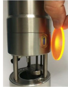
In air test of Chlorophyll a Sensor
