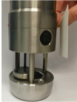
In air test of Turbidity Sensor
