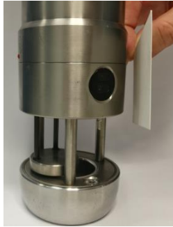
In air test of Turbidity Sensor
