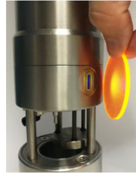
In air test of Chlorophyll a Sensor
