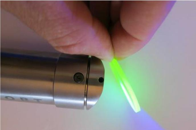
By altering the angle of the target, the magnitude of the reading should change thereby showing the correct operation of the sensor.
