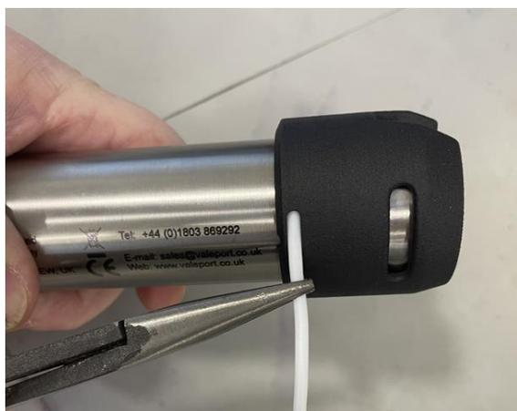
It is very tight and difficult to get all the way around the Hyperion housing. A spot of silicone grease will help.
