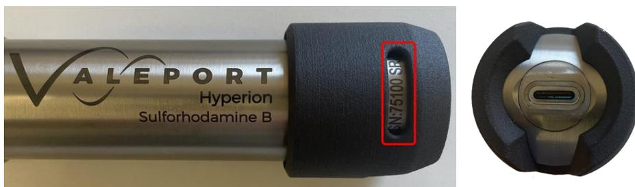
Now gently push the securing cord into the slot at the base of the guard and using a pair of pliers push the cord through the slot and around the Hyperion housing, ensuring that it is contained within the groove on the inside of the guard.
